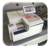
In situ saturation with humidity generator at different %HR
