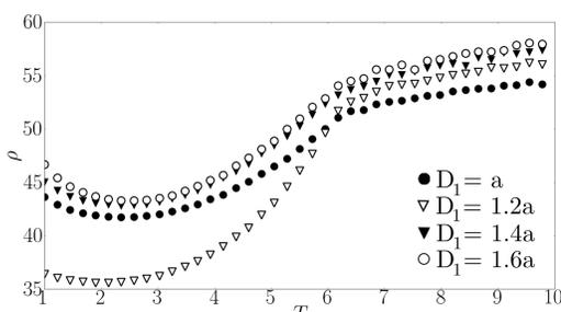
$\rho$  versus  $T$  for different values  $D_1$ . Parameter are  $J = 1$ ,  $I_0 = K_0 = -1$ ,  $D_2 = a$ ,  $n = 0.5$  one electron per cell.
