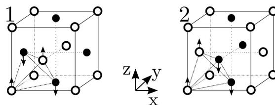
Degenerate ground state spin configurations of the FCC lattice.
